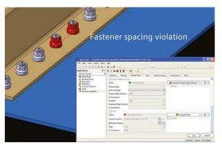
Syncrofit automatically detects and calculates the spacing between fasteners to ensure pitch requirements have been satisfied.
