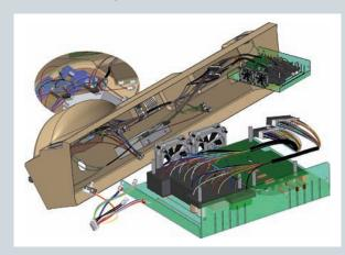
designed; live feedback immediately displays any problems. Reporting of cable and wire cut length and attributes (allowing for a slack percentage and wire stripping) are captured during the harness design process. The export of ready-to-use "net list" files adds these mechanical attributes to produce harness designs that are ready for manufacturing.
